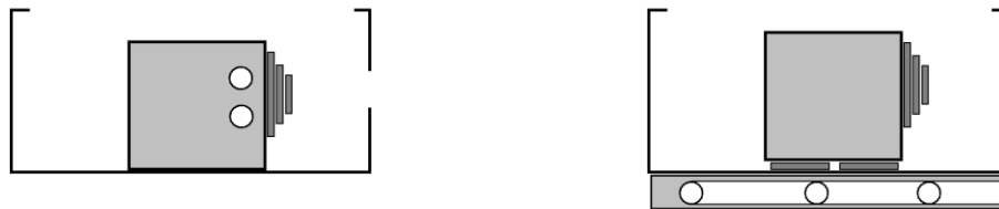
Figure 5.3: Water cooling the module. On the left, the fin-style heat sink was removed and holes were bored through the aluminum block for water cooling. The water passed directly through the aluminum block and the case. The water kept the block cool, but the desired temperature (-70 °C) could not be achieved with a single TEC stack. On the right is the heat sink configuration that is used in the final construction. In this arrangement, a two stage cooling approach is used. Heat is pumped from the 3-tier stack into the large aluminum block centered in the case. Another group of TECs is used to pump heat from this block into a water cooling block attached to the bottom of the case.
