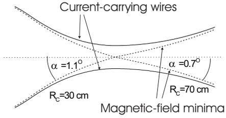
Fig. 4. Magnetic-field-minima crossing. For our curvature ( $R_c$ ) and spacing the magnetic field minima cross in the center region with an angle  $\alpha$  between the two trajectories. Atoms coupled into one guide are more likely to be transferred into the other guide when both wires carry equal currents, because of the tendency to shoot straight across the intersection.
